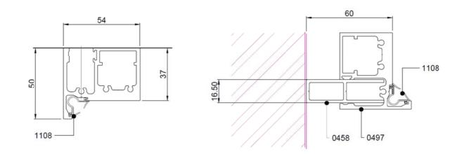
As you can see from these Designer's Guide extracts, the frame section is very similar and has simply been stretched to give it the 50mm face dimension. The standard frame widths will increase by 20mm to account for the extra girth.
